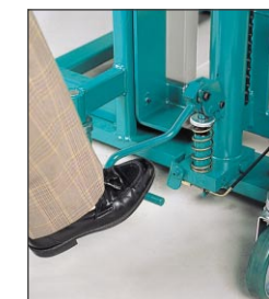
Easy Lifting by pumping pedal Pedal can be folded (Manually Operated Models)
