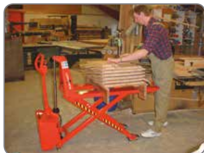
Optional extras: remote control, level control, brake, separate or built-in charger.
